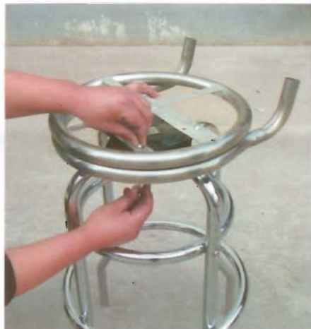
Step 5: Screw the 2-ring seat base on the top of the swivel plate.
