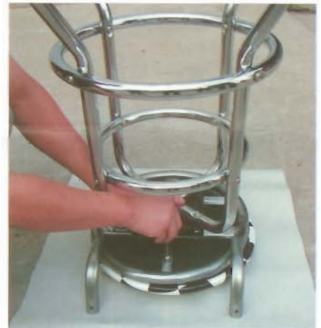
Step 6: Turn the whole barstool over, screw the 3-ring seat base to the seat pad.
