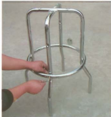
Step 2: Slide the 1st ring on over the barstool legs, bolt it together.
