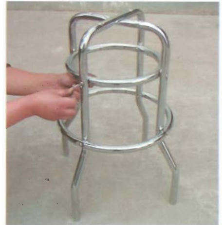
Step 3: Slide 2nd small ring inside the two legs and screw it together.
